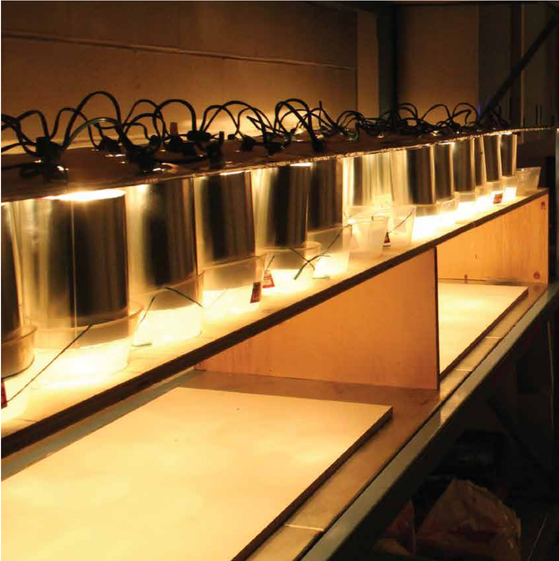
Figure A1. The Berlese-Tullgren funnel system used to extract soil invertebrates from soil cores. We used 5 W clear incandescent light bulbs in each funnel for 3 days to extract soil invertebrates. Day light intensity was kept at 50% with a dimmer switch and increased to 100% for days 2 and 3.
